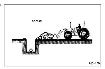
Do not use bucket in dumped position for bulldozing. This method, shown above, will impose severe shock loadings on dump linkage, bucket cylinder and tractor.
